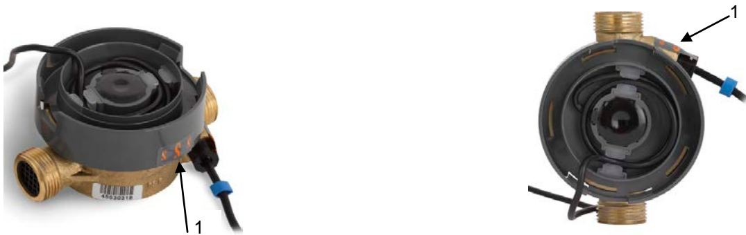
Seals installed in the factory (1) on flow meter and temperature sensor of the Supercal 739 single jet
